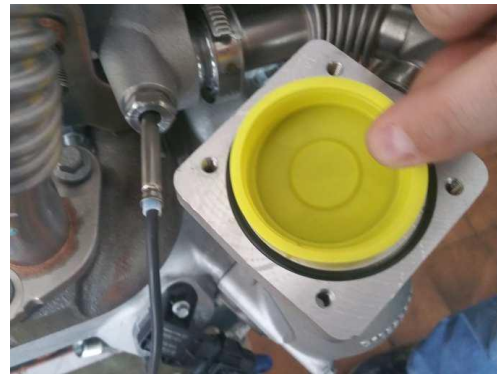
D Seal the intake elbow with an appropriate cap to prevent foreign material ingestion
